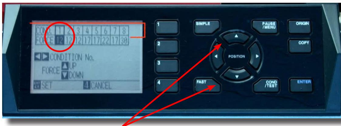
Now use the **UP/DOWN Arrow** buttons on the panel to enter in your starting force and press the **ENTER** button.
