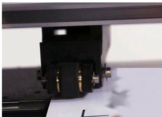
Align the **left** edge of the left roller bracket to the left edge of the paper. This placement should correspond to the blue grit-roller marks above the page load area since the edge of the page will fall on top of a grit marker.
